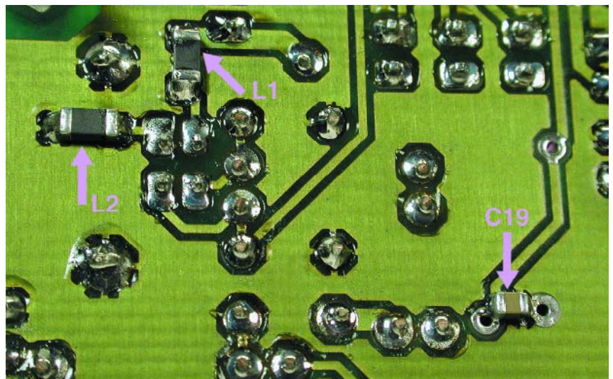
Figure 5. Just like C19, SMD chokes L1 and L2 are fitted at the solder side of the board.
