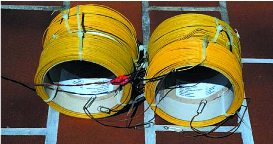
Figure 1. A receive-only antenna for the very low end of the VLF band.
