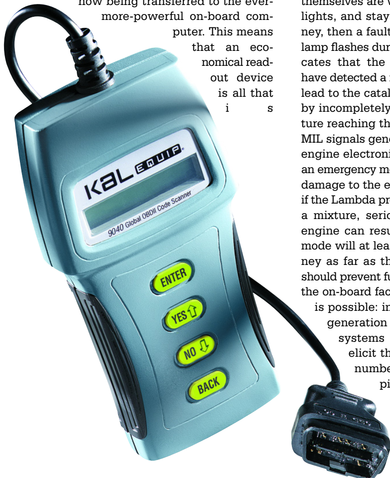
Figure 4. Typical handheld device for reading out fault codes (source: Actron Manufacturing Company, Cleveland, Ohio).
