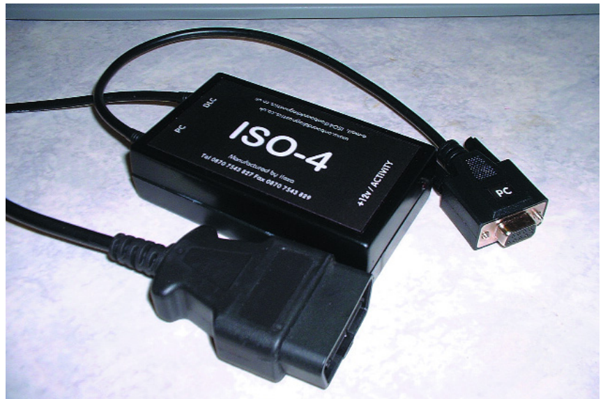
Figure 7. Elektor version of an OBD-2-to-RS232 converter. This design employs a PIC microcontroller.
