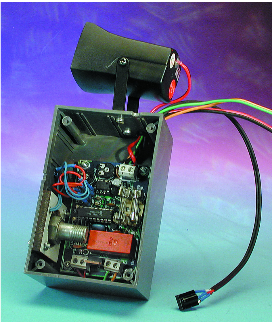
Figure 5. A view inside the prototype of the alarm. The way in which it is installed depends very much on the type of bike or scooter.
