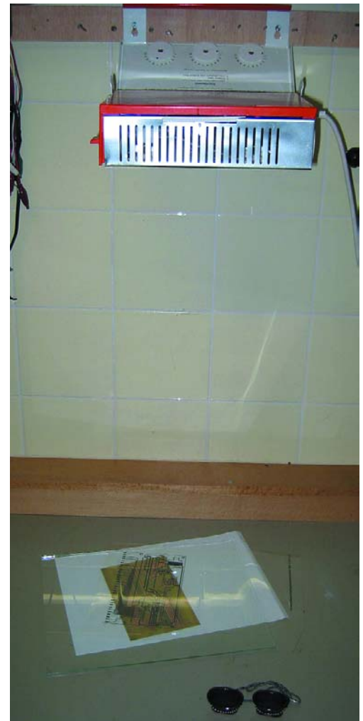
Figure 2. The exposure process using a regular sun lamp.
