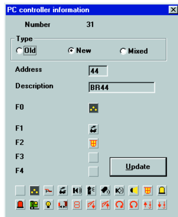
Figure 4. There are now three types of soft controller to choose from, and the address range has been increased to 255.
