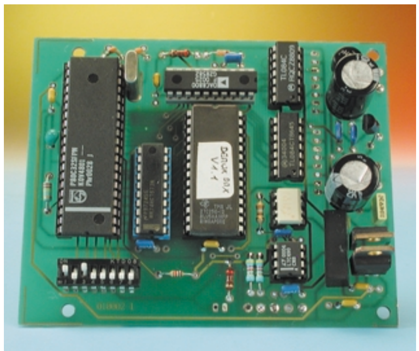
Figure 3. A fully assembled example of the DMX demultiplexer.
