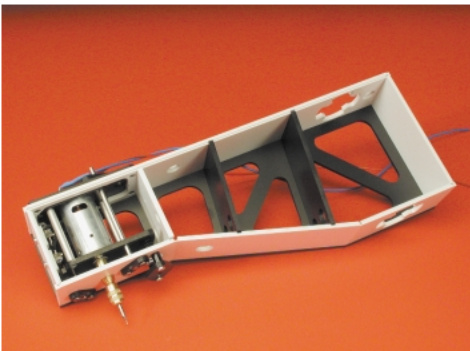
Figure 4. Tool arm, immediately before gluing of second side panel.
