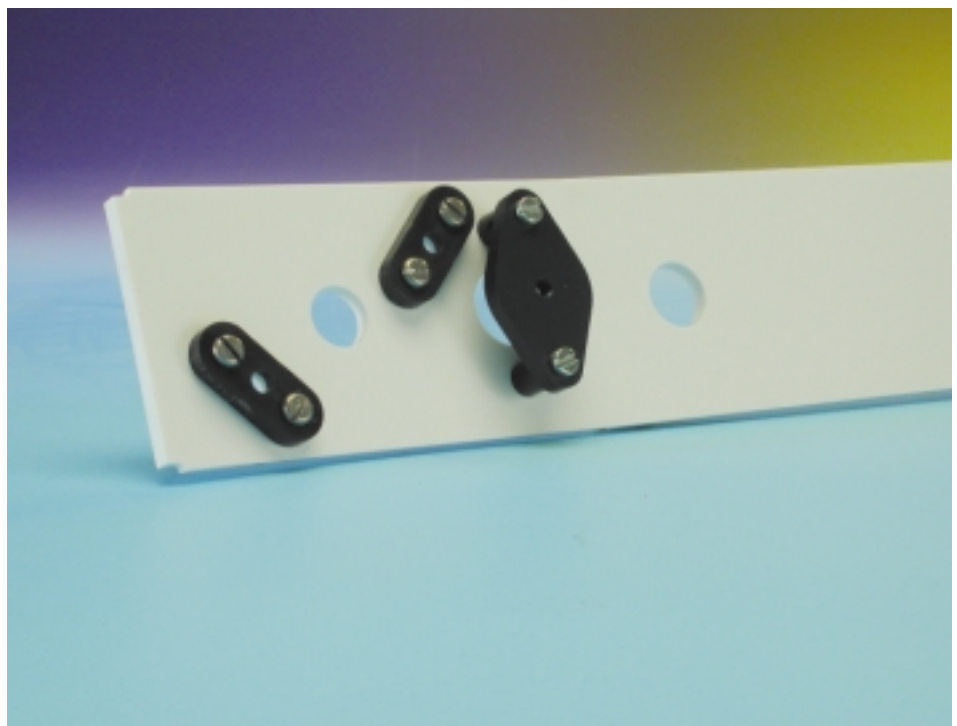
Figure 9. Bearing blocks and spring hole cover on the underside of the arm. There are two identical bearing blocks on the upper side.
