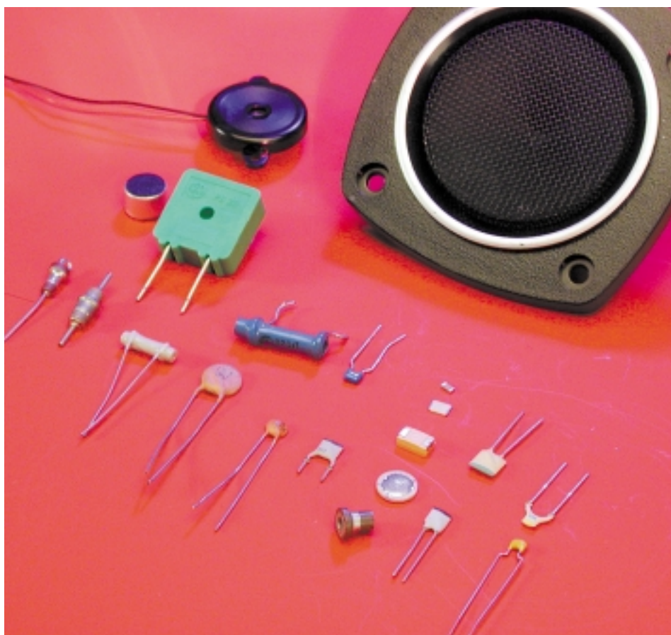
Figure 8. Some electronic components made from ceramic substances. The front row shows a selection of RF capacitors.
