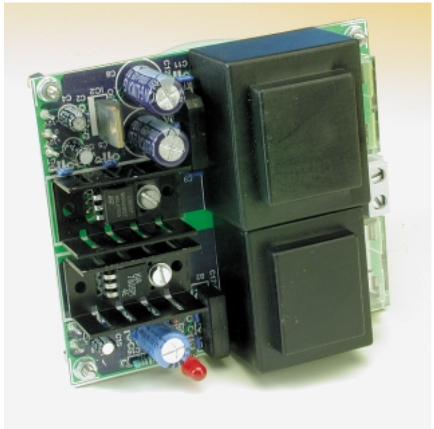
Figure 5. Small heat sinks must be provided for voltage regulators IC1 and IC3.
