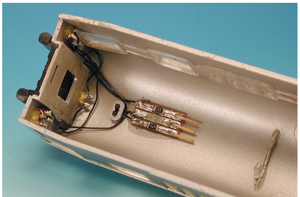
Figure 7. Connecting the front and rear signal lamps.
