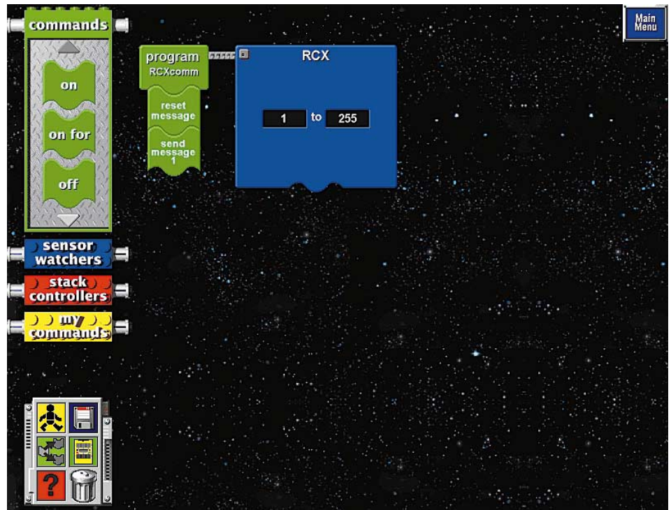
Figure 1. The icons belonging to the message functions in the Lego software.
