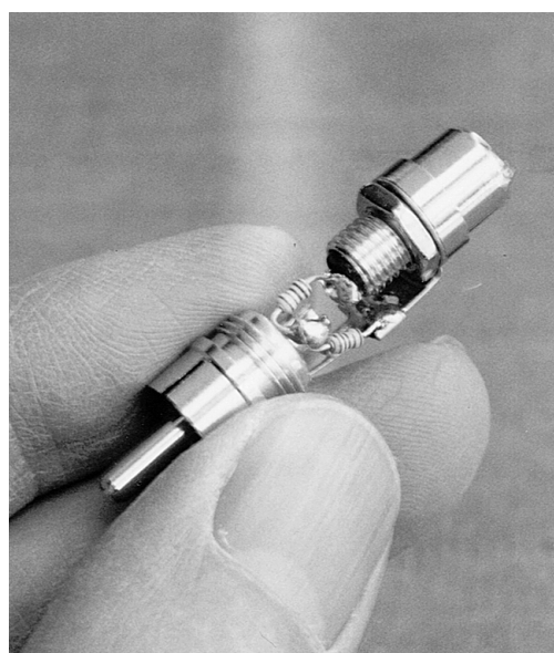
Figure 3. A Cinch plug and cable jack can be used to make a handy in-line connector with a built-in attenuator.
