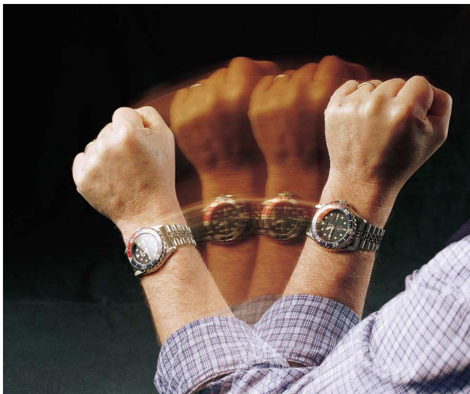
Figure 1. In both 'automatic' and 'kinetic' watches, kinetic energy is converted into stored energy for operating the clockwork. No batteries needed!
