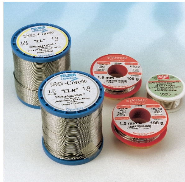
Figure 2. A few samples: the large rolls hold wire solder made from the eutectic tin/silver/copper alloy Sn95.5Ag3.8Cu0.7. They differ only in the flux content (3.5% for normal use and 1% for SMD soldering). The smaller rolls hold wire solder made from tin/silver (Sn95Ag5) and tin/copper (Sn99Cu1) alloys. The smallest roll is once again a tin/silver/copper alloy.
