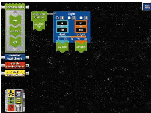
Figure 5. The RCX module can be completely configured using this screen. The operating system is also downloaded to the RCX module using the menu.
