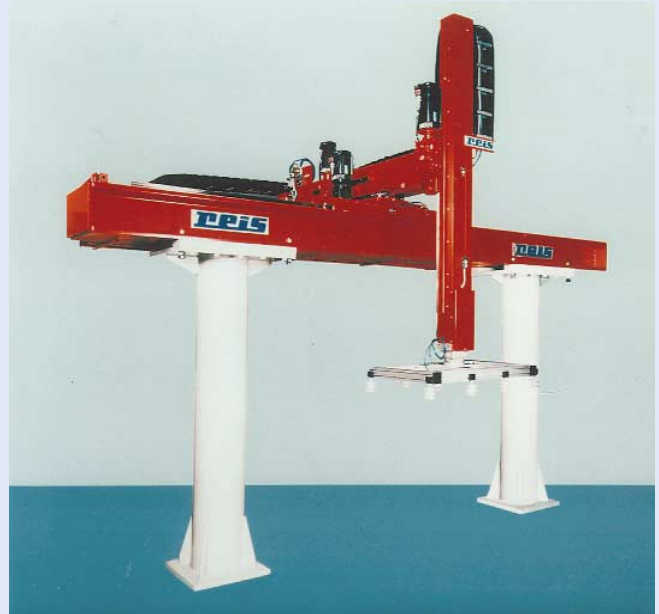
Figure 2. Linear teleoperator with three translational joints.
