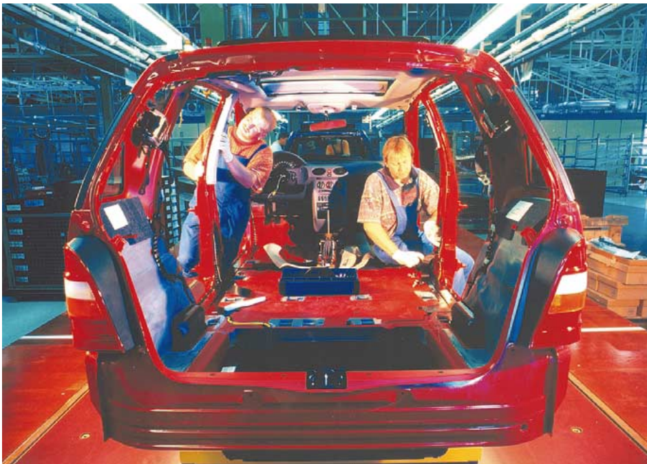
Figure 3. Owing to customers' requirements, completion of the interior of the car requires more workers than robots, that is, this stage is more labour intensive than the remainder of the car.
