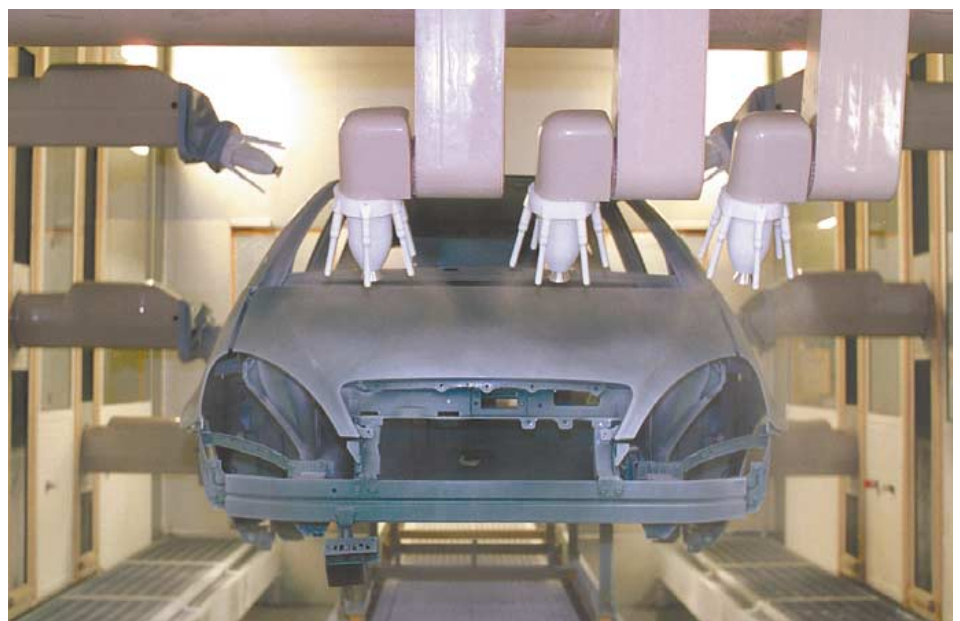
Figure 2. Application of the final (clear) solvent-free lacquer by a paint robot.
