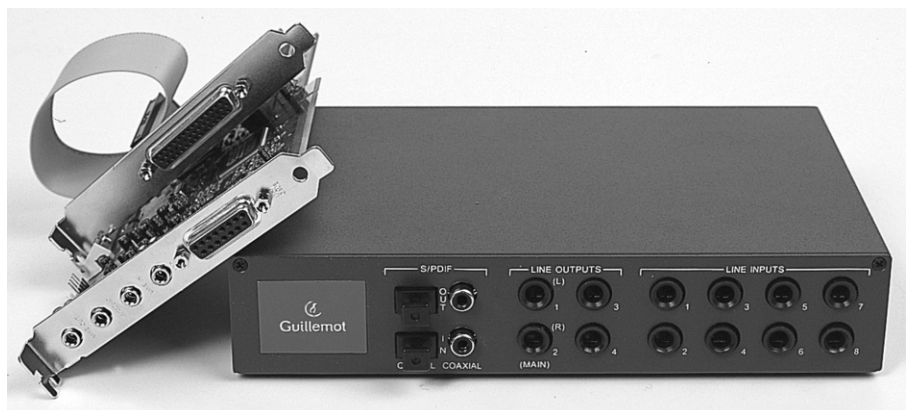
Figure 3. This card from Guillemot provides a handy setup for the true audio hobbyist, since it has all connectors and the converters located in a separate enclosure (photo: Guillemot).
