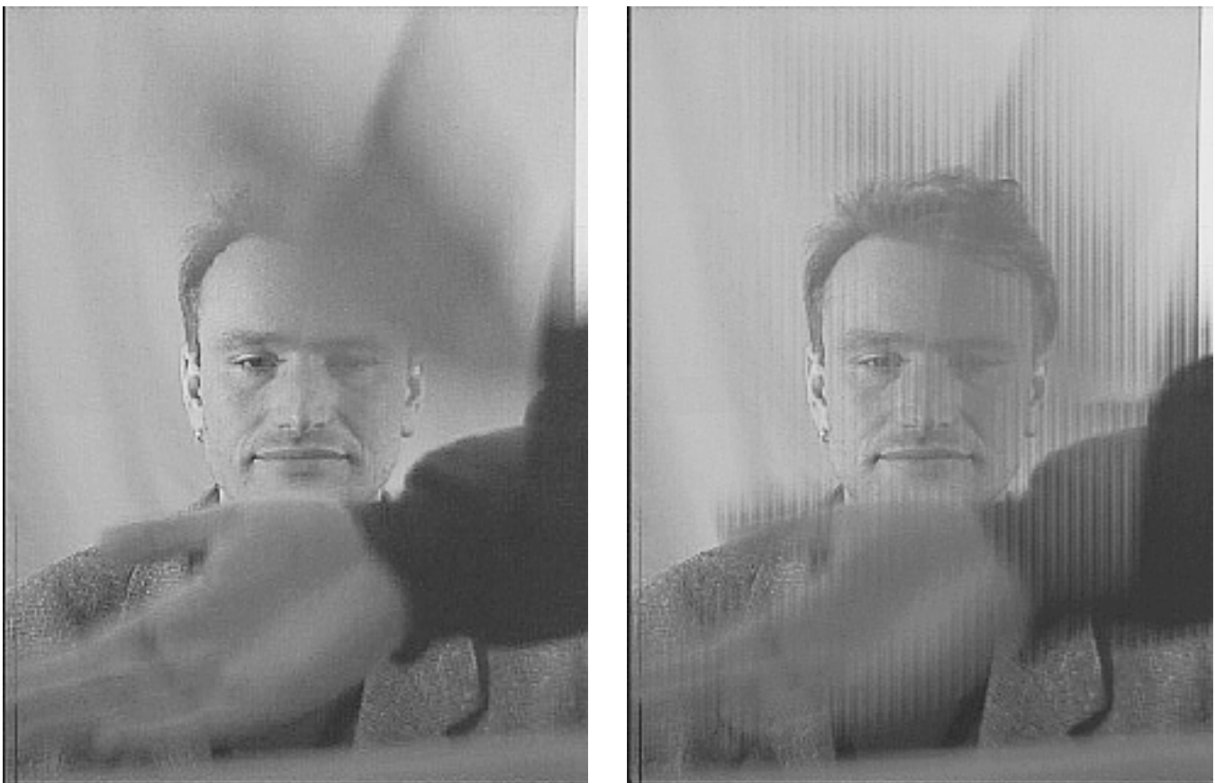
Figure 2. An example of the comb effect. In this recording of a speech, the missing clapperboard was replaced by a handclap. Left: no comb effect, right: comb effect
