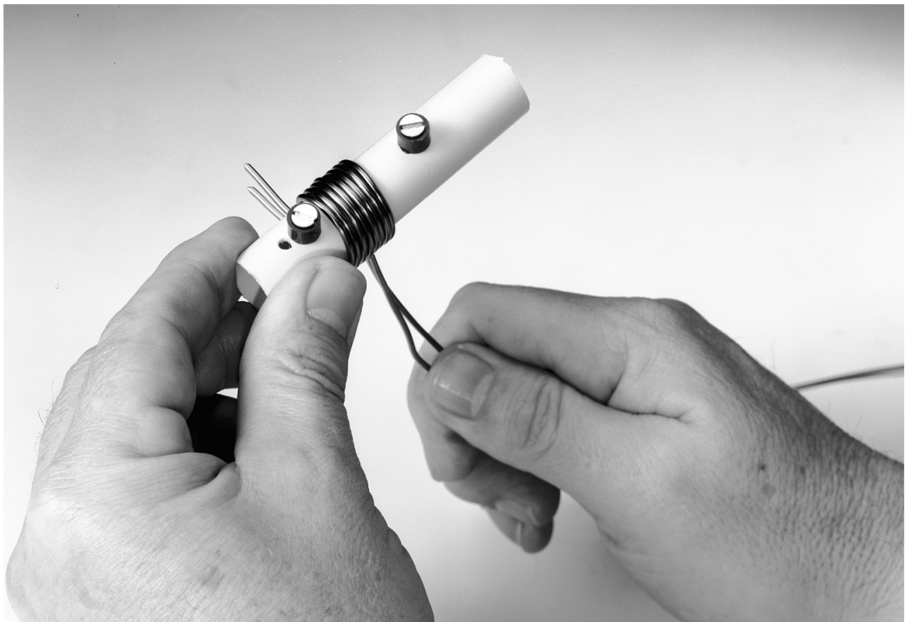
Figure 14. Air-cored inductor L_1 is formed by laying two windings each of eight turns of doubled-up each on top of one another. The former is a length of 16 mm diameter PVC pipe as used by plumbers. The resulting four windings are simply connected in parallel.
