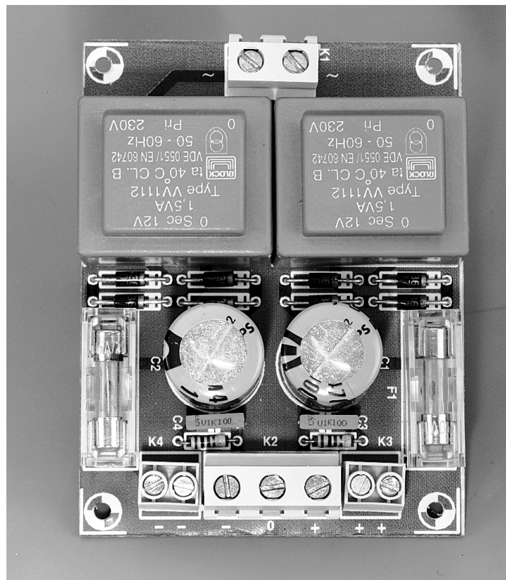
Figure 8. The auxiliary power supply is small enough to fit in most enclosures.
