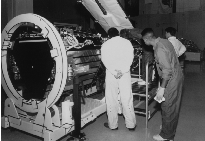
Figure 2. Assembly of the nearly 700 kg weighing satellite at the Motorola-SATCOM plant in Chandler, Arizona. Note the triangular cross-section of the carrier structure which is made of reinforced man-made fibre.
