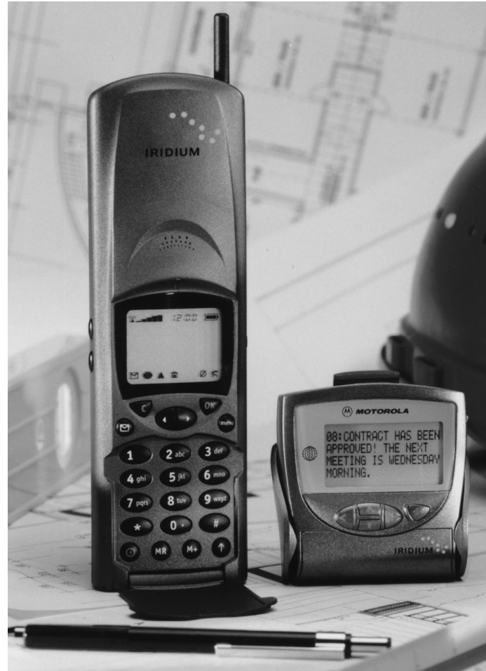
Figure 4. Iridium pager and mobile phone from Motorola. The phone has an interchangeable frequency module for a number of mobile phone standards and needs an additional L-band antenna unit for operation in the Iridium Network.
