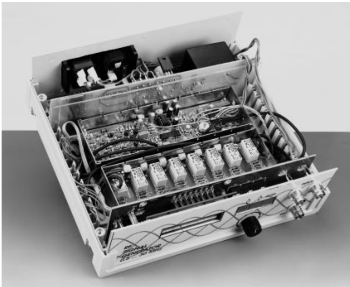
Figure 13. A look inside our prototype of the RF Signal Generator. The covers of the tinfole cases of the VFO/PLL board and the attenuator board were removed for this photograph.
