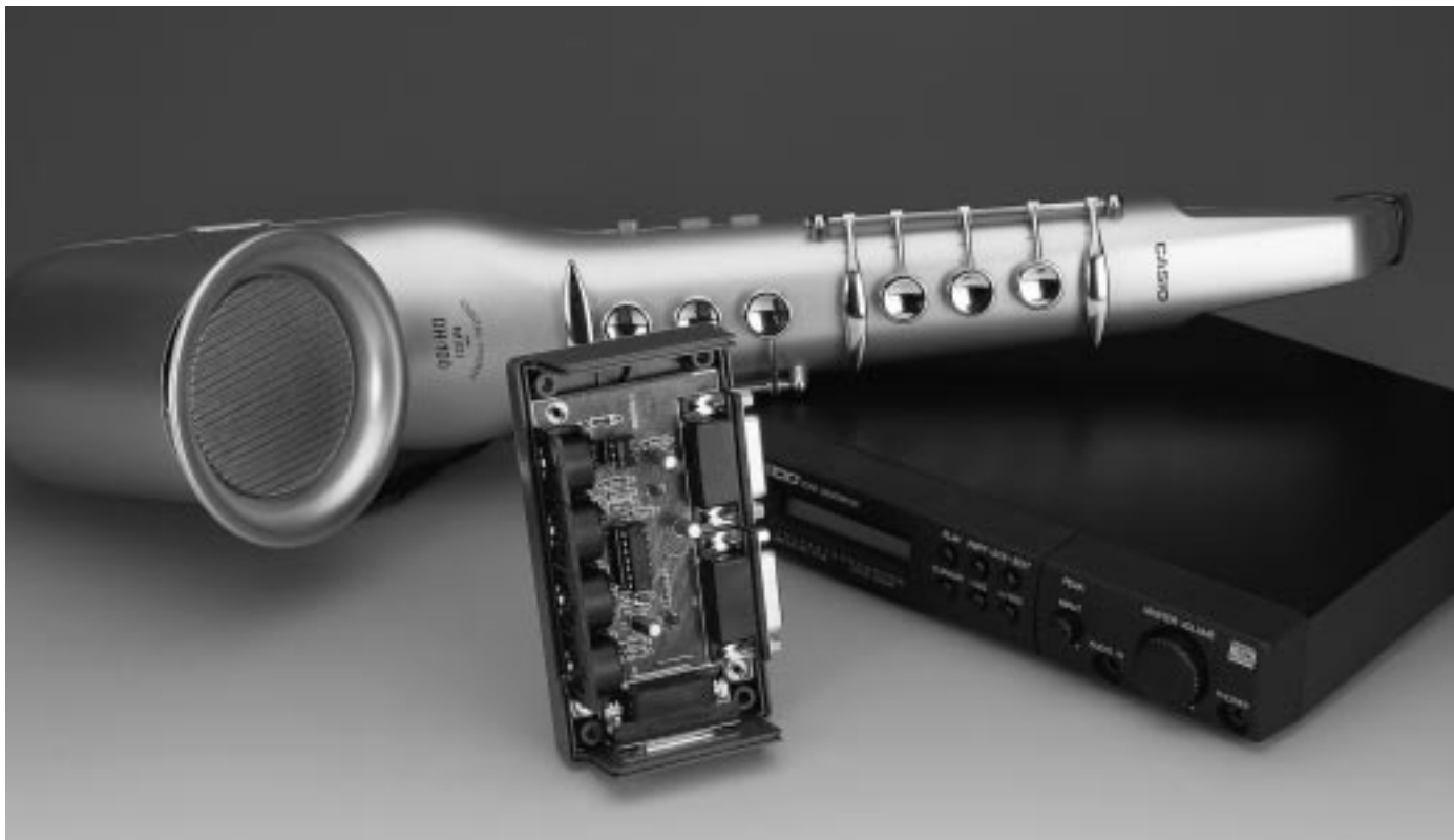
Figure 4. The MIDI connections allow commonly used MIDI instruments to be hooked up, like this expander from Yamaha, or Casio's electronic saxophone.
