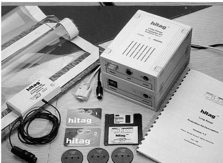
Figure 9. Evaluation and demonstration kits of RFID systems are available from several manufacturers. Those shown are from Philips/Mikron.
