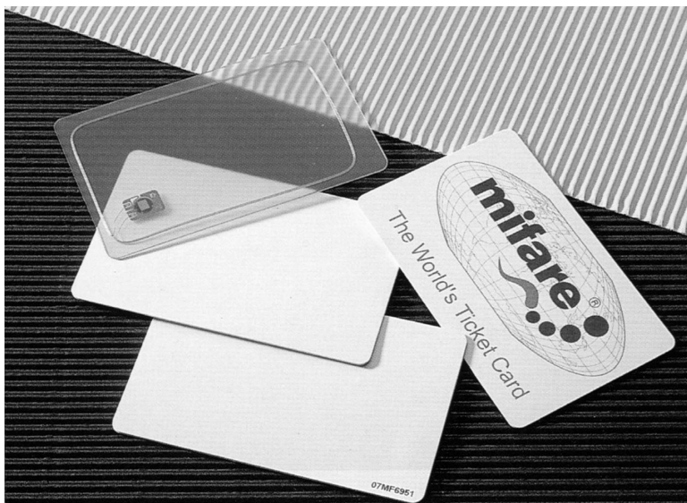
Figure 5. This contactless smartcard is the data carrier of the Philips/Mikron Mifare® RFID system designed for electronic ticketing. The card is suitable for use in public transport, parking meters, electronic keys, road tolls, ID cards, and more.
