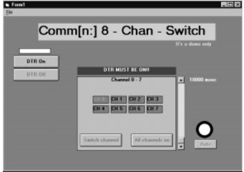
Figure 5. The user interface is a window with buttons offering full control over the eight switched devices, as well as useful status information indicators.
