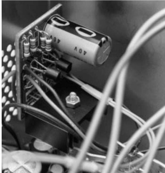
Figure 5. Here you can see how the regulator circuit can be built into a PC power supply.
