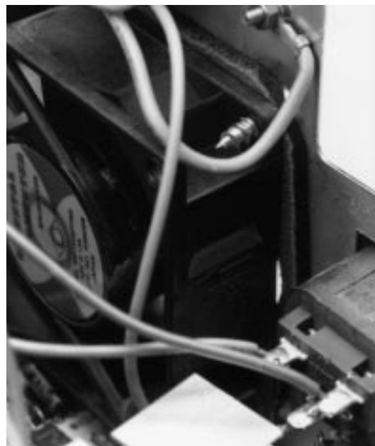
Figure 2. A rubber ring mounted between the fan and the enclosure can significantly reduce the amount of vibration which is coupled from the fan to the enclosure.
