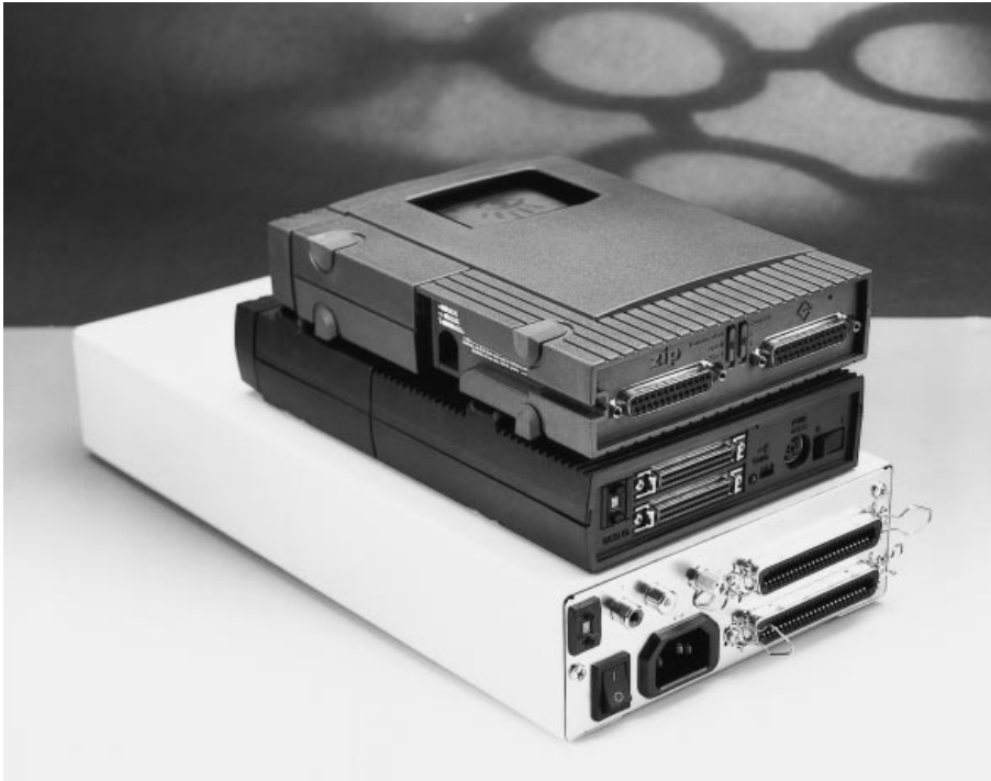
Figure 3. The rear panels of three external SCSI devices (Zip and Jaz drives, and a CD-ROM player). The differences in the connectors can be clearly seen. Also note the switches for setting the device identifier numbers
