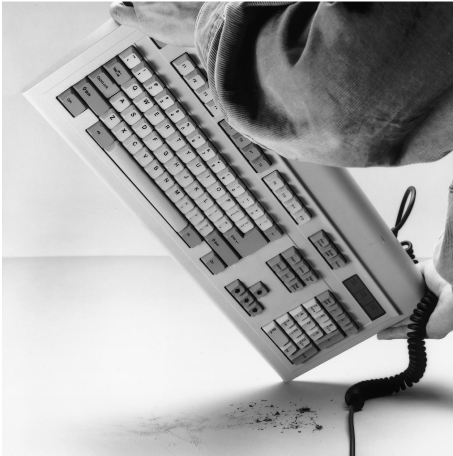
Figure 7. Illustrating the keyboard shake-out. You'll be amazed at the amount of debris lodging in a PC keyboard.
