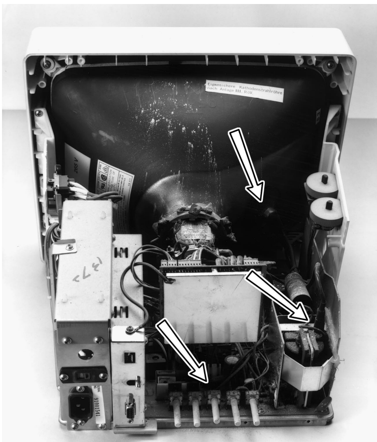
Figure 8. Internal cleaning of a PC monitor should not be attempted by beginners. The arrows in this photograph point at spots which are likely to be covered in dust.
