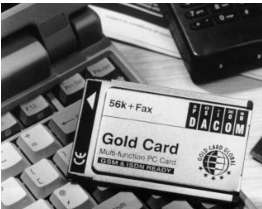
Figure 7. A number of manufacturers have 56 kbit/s modems available. These normally use chipsets from Lucent, Rockwell or US Robotics.
