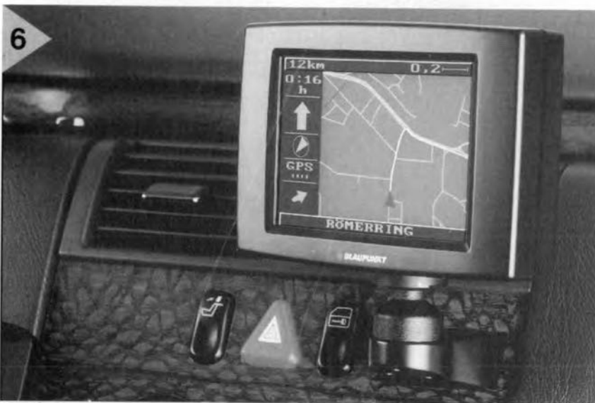
Figure 6. It is possible to show a diagram of the route guidance on the electronic map on the LCD monitor.
