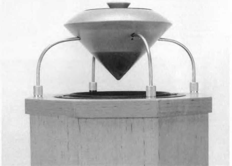
Figure 5. Side view of the cone construction. Two of the brass clips are used as terminals for the tweeter.
