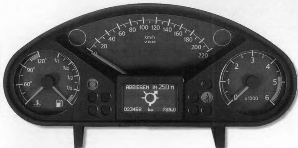
Figure 3. Navigation display in a combined dashboard instrument from Mannesmann-VDO, which is linked to a central computer.
