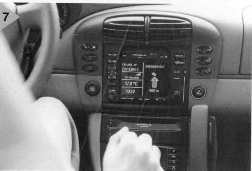
Figure 7. The integrated driver information system (IDIS) from Siemens includes the control of the vehicle's audio system, mobile telephone and on-board computer. This system is offered as an optional extra on Porsche cars under the name Porsche Communication Management (PCM).
