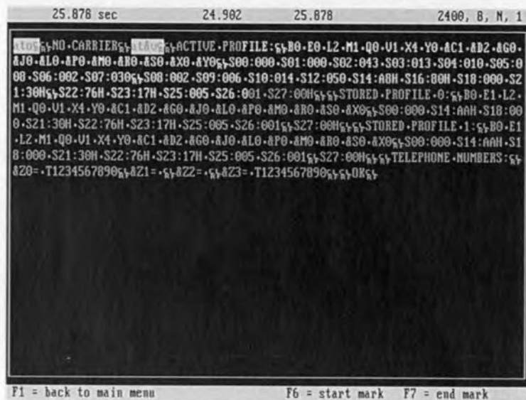
Figure 1. The "ASCOPE" program measures asynchronous (RS232) signals and displays them on the screen of the monitor. Afterwards, they may be saved as a data file.
