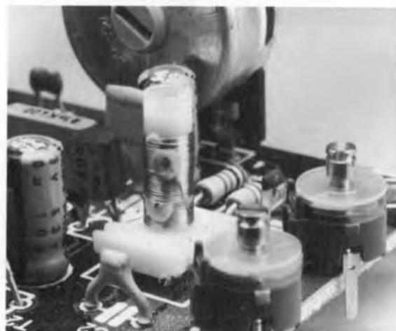
Figure 4. Close-up of the finished input band filter, L1-L2, fitted in the circuit. Do not apply too much heat while soldering the enamelled copper wire, as the 10F1 base is prone to soften a little and the pins will easily come loose. Also note that we've used a few drops of candle wax to secure the windings.
