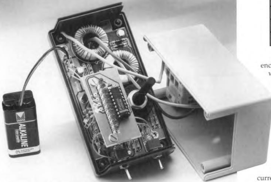
Figure 3. Photograph of the completed prototype. Note that the earth wire should be continuous from entry plug to trailing socket.
