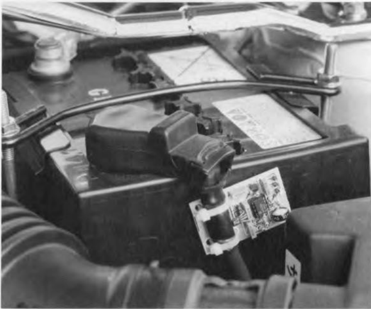
Figure 2. The battery current is measured with the aid of a magneto-resistive sensor; there is no need of interrupting any circuits.
