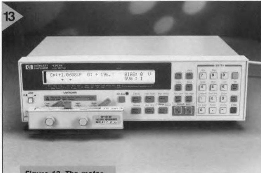
Figure 13. The meter is compared in the text with this Hewlett-Packard LCR meter, which is, however, not affordable by the average amateur.
