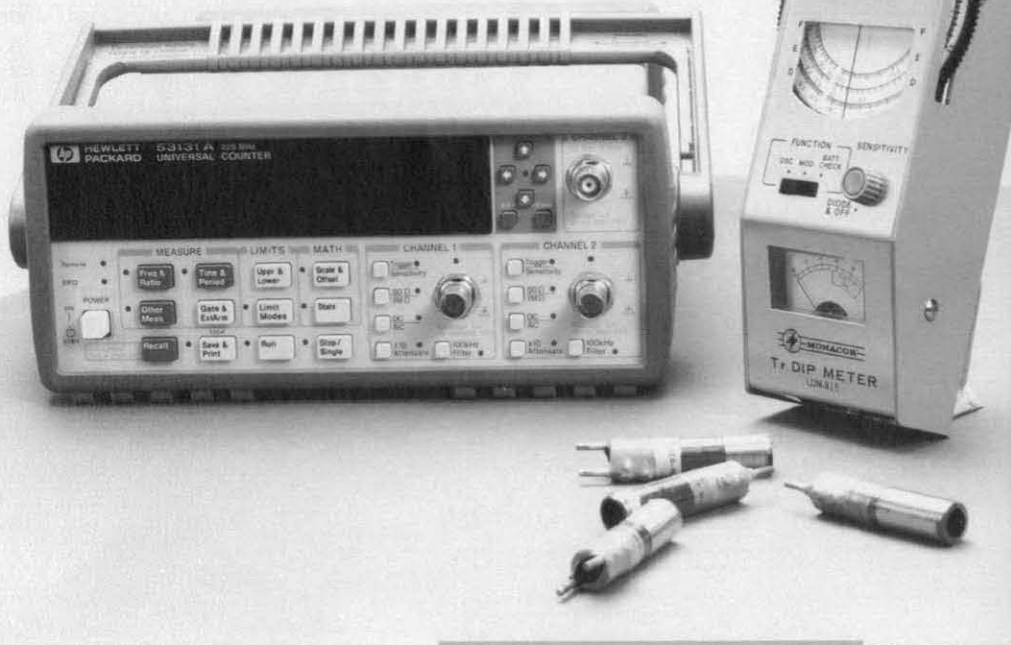
Figure 5. A frequency meter is a very useful instrument, but for many test purposes a dipmeter is a much cheaper alternative.
