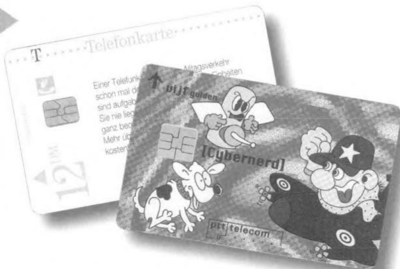
Figure 2. On these phone cards, the chip is in the ISO position.
