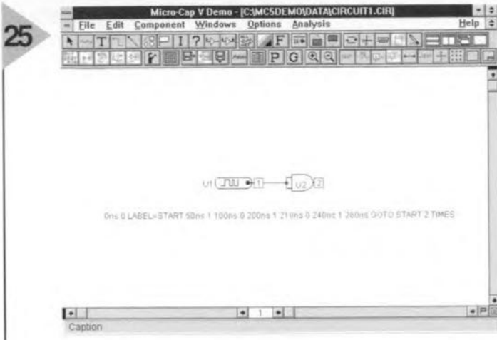
Figure 25. Simple beginnings: one digital signal generator sending a one-bit signal to one logic gate.
