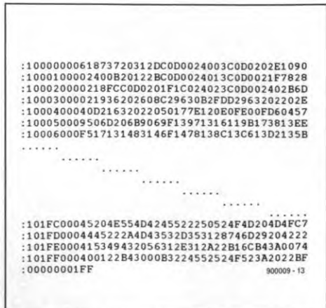
Fig. 2. Hexdump of the start and end of the Intel-hex file sent by the BASIC computer.
