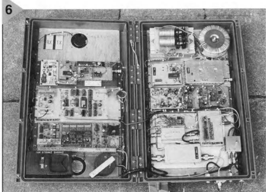
Figure 6. What do you mean home construction is on the decline? Pictured here are the electronics of a 23cm-in/13cm-out cross-band ATV repeater station, PI6ANH, which was recently taken into use. The QTH of this station is JO21XW, ERP is about 50 W, and the antenna height is 40 m a.s.l. A wonderful example of high-end equipment built and operated by radio amateurs, this repeater is one of dozens located at elevated sites all over Europe. PI6ANH even has its dedicated Internet site at http://www.regio.rhein-ruhr.de/hamradio/atv .
