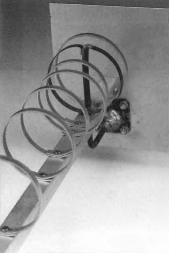
Figure 5. The best known antenna for 23-cm ATV use is the loop yagi. Pictured here is a home-made loop-yagi scaled for 13 cm (courtesy Rob, PE1CHY).
