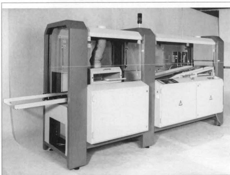
Fig. 4. Wave soldering is a technique applied with leaded components, but also with SMDs (photograph courtesy Ersas).
