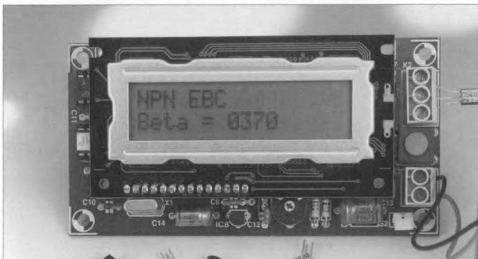
Fig. 6. Normal test result for an n-p-n transistor with emitter (E) at pin 1 of K_2 , base (B) at pin 2 of K_2 , and collector (C) at pin 3 of K_2 . The current amplification factor, \beta = 370 .
