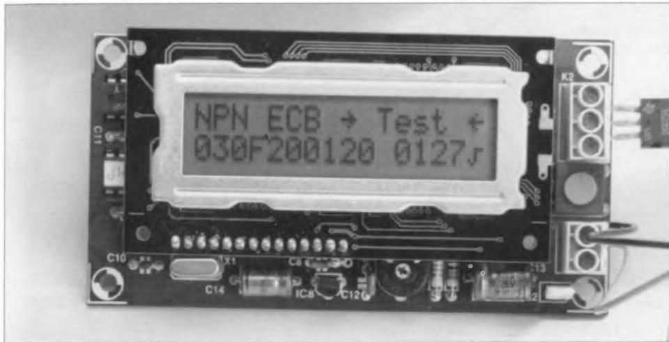
Fig. 8. In the single-step mode, the result of the test performed during the previous cycle is displayed. Note radical sign after '0127'.
