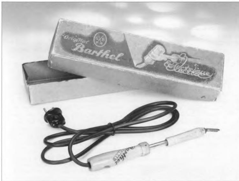
Fig. 2. When it comes to soldering, the soldering iron is the best known tool for the trade. This vintage type was introduced in the fifties, and is not really suitable anymore for soldering modern circuits. Note the burnt edges of the cardboard box onto which the iron was occasionally landed.
