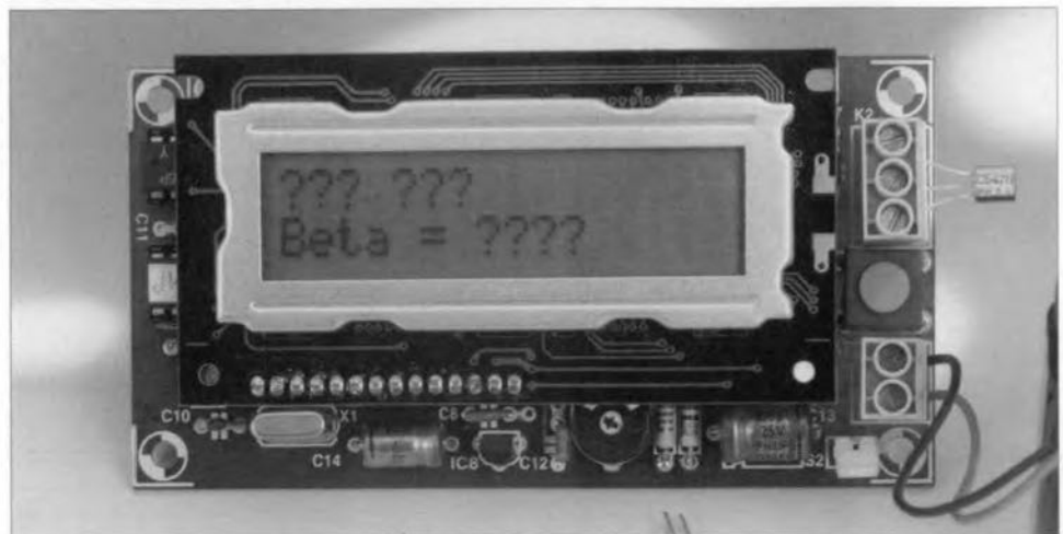
Fig. 7. This error display appears if the test results are not realistic. This may not necessarily mean a faulty transistor: it may indicate that \beta > 1000 .
