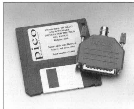
Fig. 5. This adapter from RS Components enables laptop and palmtop computers having only the standard interfaces (such as printer port) to be used for measurements. Great for field work and servicing! The software is supplied by Pico Technology.
