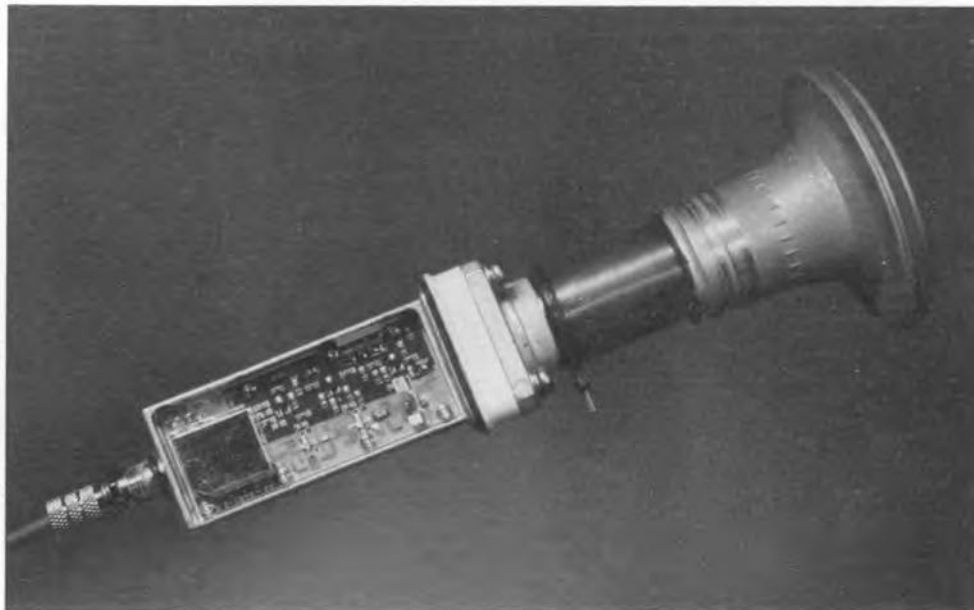
Fig. 1. Typical HEMT LNB with magnetic polarizer. The plastic cover around the polarizer was removed for the purpose of this photograph. Inside the LNB, the HEMT input transistor is located underneath the small screening fitted upright on the PCB.
