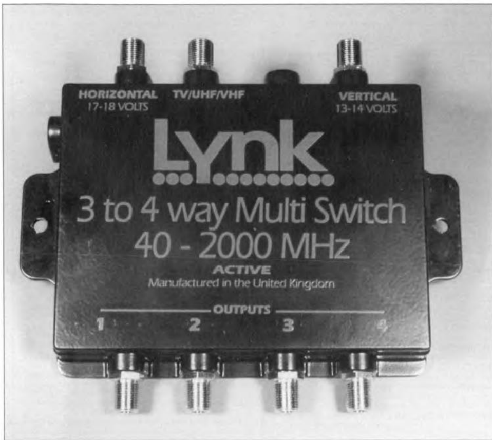
Fig. 8. An active four-way switch with optional insertion of terrestrial (VHF/UHF) TV signals. LNB signals are applied separately for the two polarization planes, for which the Multiswitch supplies the appropriate supply voltages.
