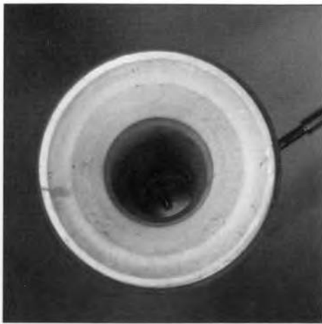
Fig. 4. A quarter-wave probe is used to couple the RF signal from the waveguide to the input of the LNA. Obviously, the polarizer was removed from the LNB input for the purpose of this photograph.
