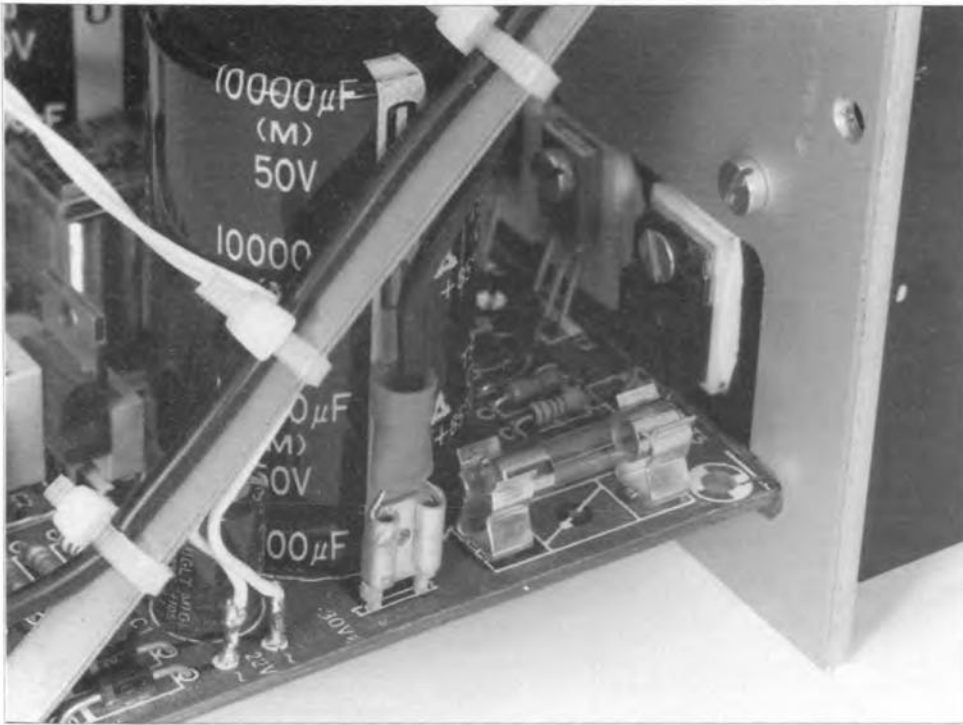
Fig. 10. Car-type flat connectors are ideal for use with large currents.
