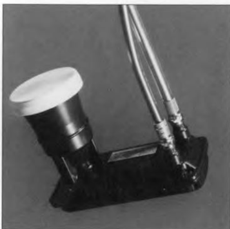
Fig. 5. A 'twin' LNB: two mutually independent V/H converters with a shared microwave fed system in a single case. Ideal for two satellite TV receivers on a single dish.
