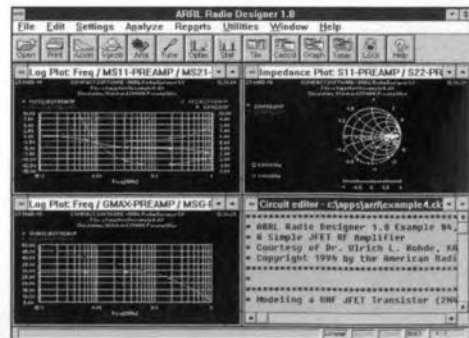
Fig. 9c. Circuit editor and all three (pre-defined) reports on a simple JFET preamplifier (example).
