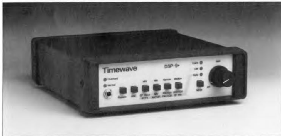
Fig. 10. The Timewave DSP-9+ is a highly intelligent and technically very advanced 'noise killer' for a multitude of radio modes including SSB, CW, RTTY, AMTOR, PACTOR, HF packet and G-TOR. Based on a digital signal processor (DSP), the unit is simply connected to the earphones socket of your receiver or transceiver.
