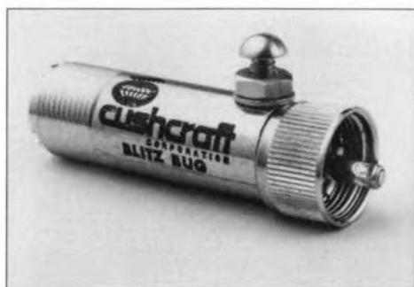
Fig. 8. The Blitz Bug from Cushcraft is based on a patented three-point static discharge design. The device features a sealed air chamber, constant static drain, and controlled voltage discharge. The Blitz Bug is rated at 2 kW PEP to 500 MHz with negligible insertion loss. Shown here is the LAC-1 version with UHF PL-259 and SO-239 connectors.
