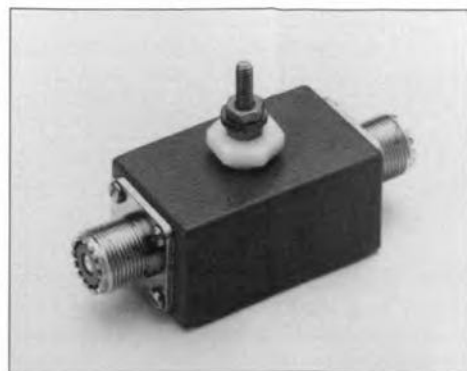
Fig. 7. Protect your valuable equipment from surges up to 5,000 ampères with a Cushcraft constant-impedance LAC4 arrester. The LAC-4 has a replaceable gas discharge tube which clamps voltage surges to less than 50 volts in about 100 nanoseconds, much quicker than the voltage rise time of lightning.
