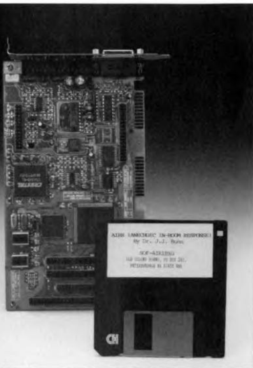
Fig. 6. These days it is possible to do pulse response, frequency response plotting and distortion measurements 'on a shoestring' with the aid of programs like AIRR and PC Audiolabs, which use the PC's internal sound card.
