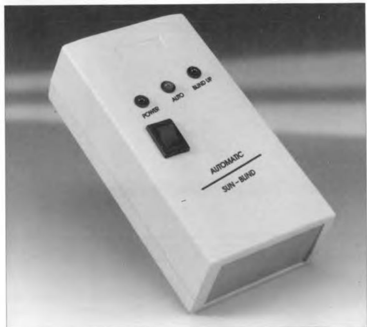
Fig. 1. General view of the sun blind control unit.
