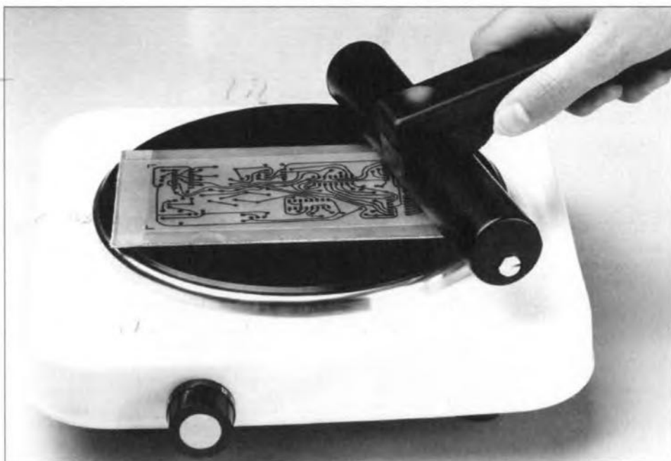
Fig. 2. Transferring the toner from the TEC200 foil to the copper-clad side of a piece of circuit board requires some pressure and a board temperature of about 140 °C. Here, a simple thermostatically controlled hotplate is used.
