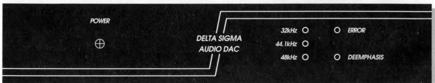
Fig. 6. Suggested front panel for the D/A converter (not available ready made) (scale 3:4).
