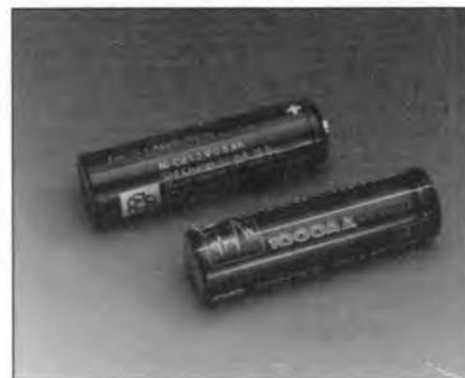
Fig. 4. The capacity of a NiMH battery is almost twice as high as that of a standard NiCd cell. The heat is on again, however, with the introduction of Panasonic's new 1,000-mAh NiCd 'UM3' size cells.
