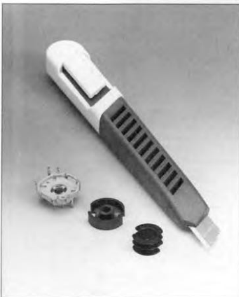
Fig. 4. Only half a pot core is used to make inductor L_1 . The double-section bobbin is cut in two with a sharp hobby knife.
