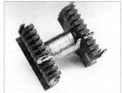
Fig. 10. This is how Tr_1 looks after the first secondary winding has been laid.
