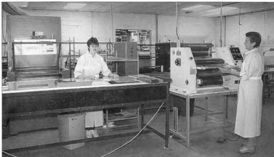
A laminate is used to apply a photosensitive layer on to the printed circuit board.
