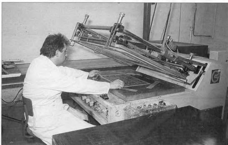
Silk screen printing is used to put the solder mask on the PCB.
