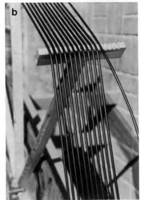
Fig. 19. Coaxial cable 100 kHz loop: (a) schematic. Note that the centre conductor of the far end is connected to the shield at the feedpoint; (b) close up.
