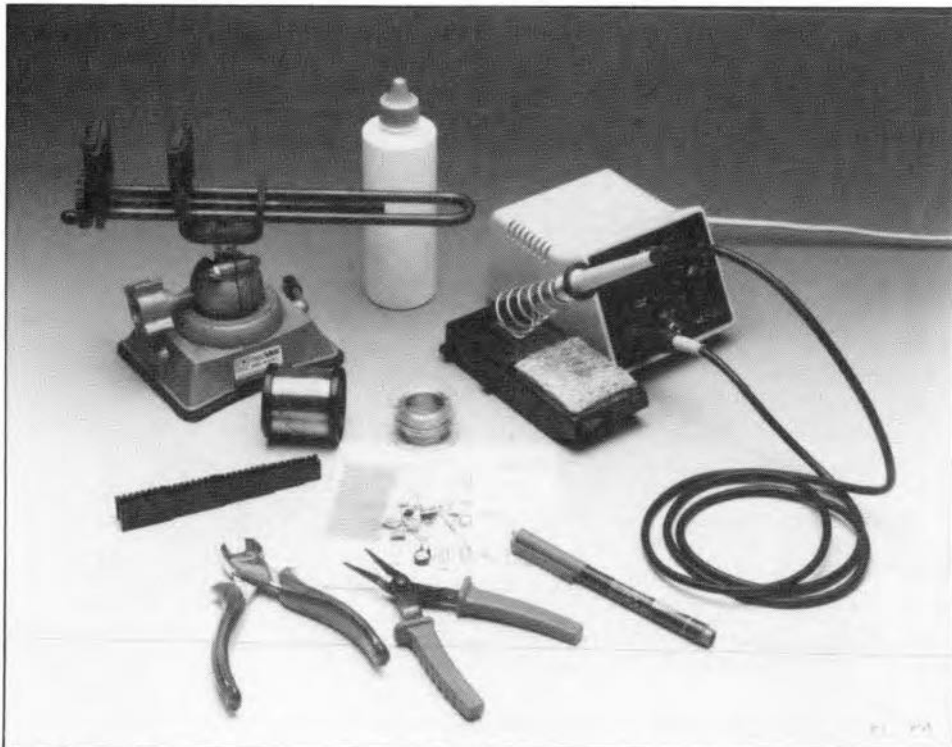
Fig. 2. Most of the tools necessary for working with prototyping board will be available in your toolcase. A water flask, a component wire preforming tool and a circuit board holder are optional to make construction easier.
