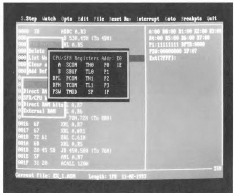
Fig. 2. The Watch menu enables you to peek inside the 8051, and see what is happening to the SFRs and the CPU.
