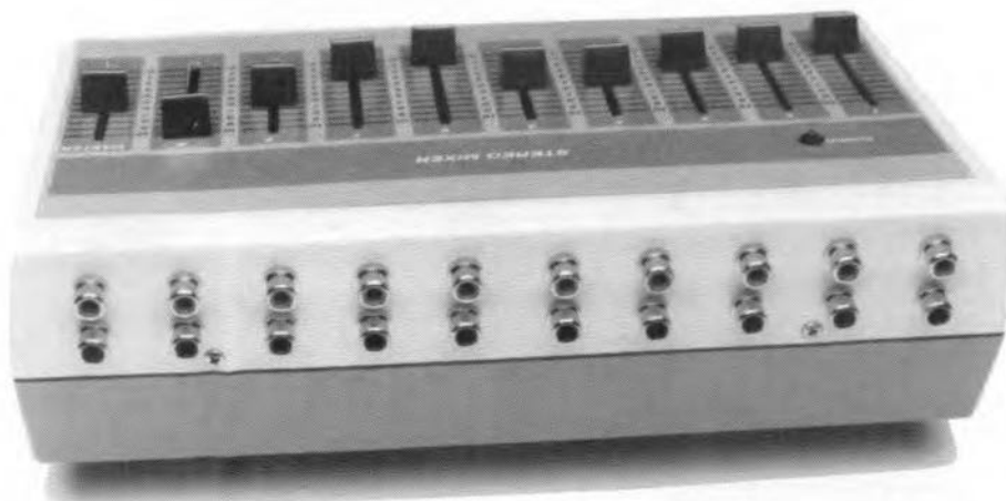
Fig. 7. Recommended way of mounting the audio sockets on the rear panel.
