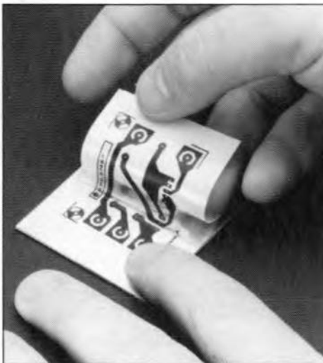
Using Letraset 'Letracopy' self-adhesive transfer film to prepare a piece of photosensitive circuit board for UV light exposure.
