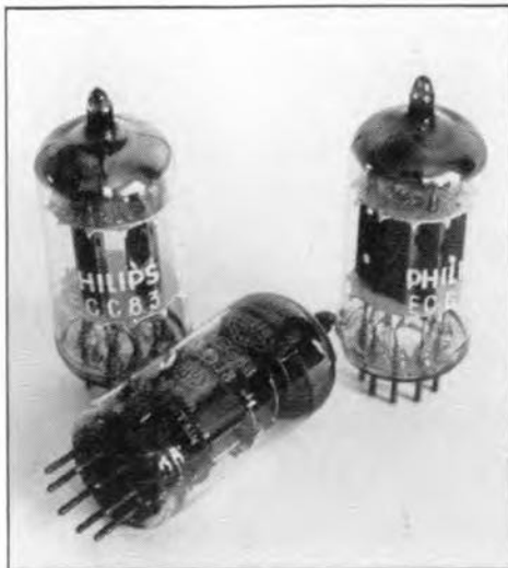
Fig. 5. Three modern all-glass dual triodes.
