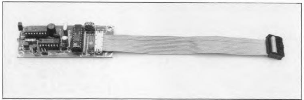
Fig. 12. The IR receiver is hooked to the Z80 card via a length of 14-way flatcable fitted with an IDC socket at one end, and an IDC plug (for PCB mounting) at the other.
