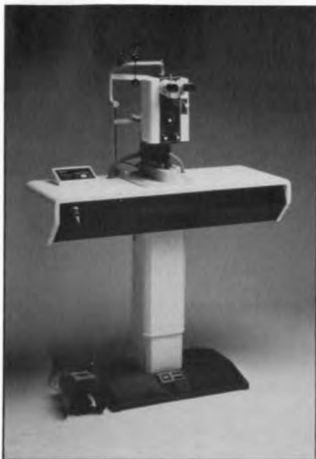
Fig. 7. A clinical argon laser, primarily used for retinal photo-coagulation.
