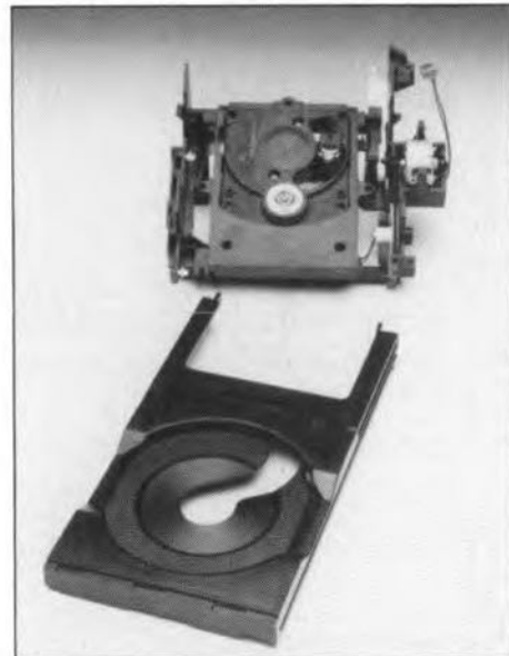
Fig. 4. Disk compartment removed from deck.
