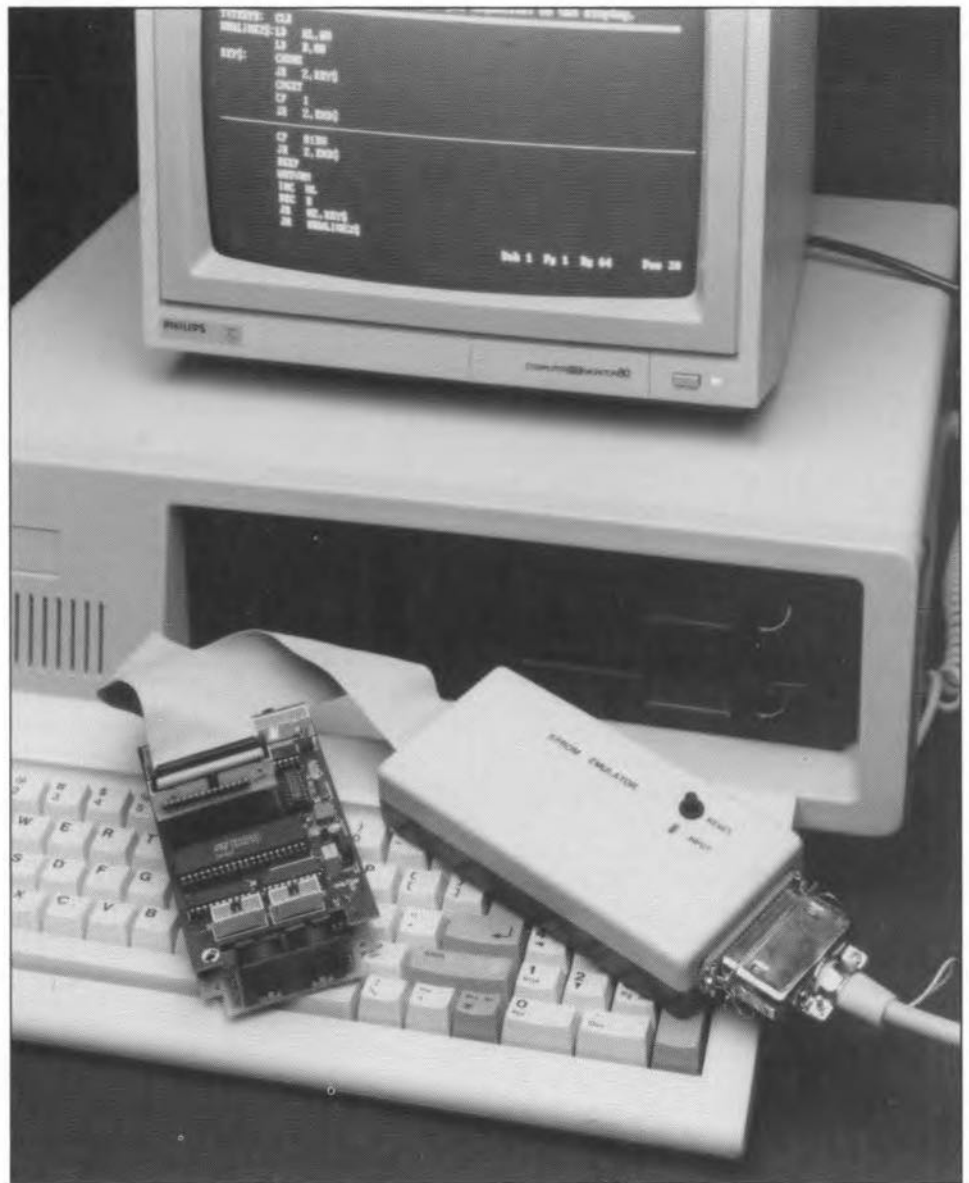
Fig. 4. Undoubtedly the most flexible way of developing software for the Z80 board is by means of an EPROM emulator and a PC running a Z80 assembler.
