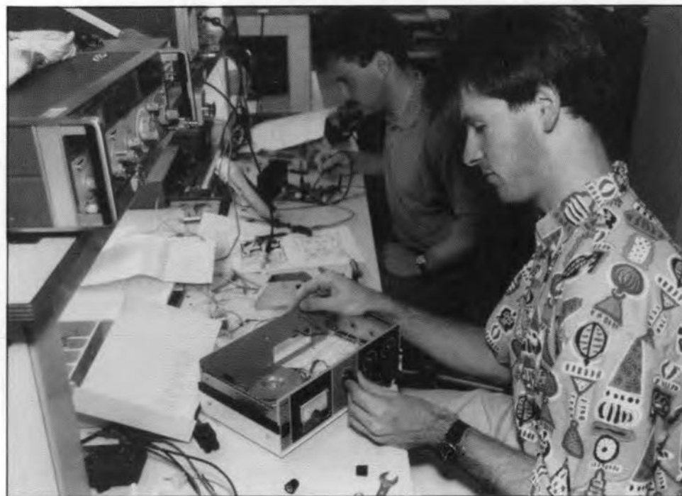
Fig. 4. Preparing the enclosure and the front panel before the PCB is fitted.
