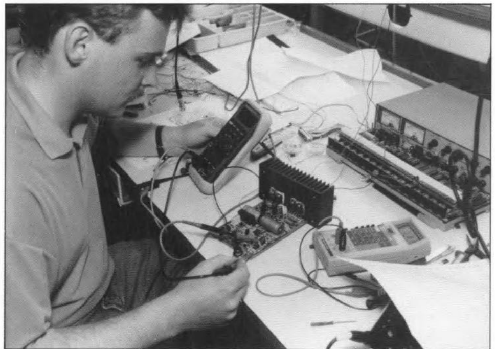
Fig. 3. Initial test on the assembled board.
